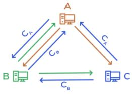
Now, as Alice and Bob both know that Chuck is the adversary, each of them creates a special proof-of-fraud transaction, accusing Chuck of fraud, with both signed hashes of Chuck's sets ( $hC_A$  and  $hC_B$ ) attached as a proof, and adds it to the transaction set. If the shardblock proposed by Alice and Bob wins the consensus round, Chuck's stake is slashed.
