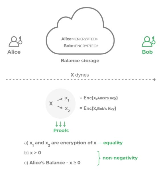
Instead of subtracting x from A and adding x to B, roughly speaking, we subtract encrypted x from encrypted A and add encrypted x to encrypted B.
